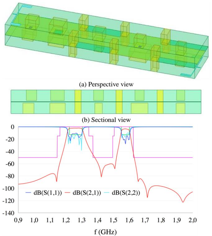
Figure 4. Filter model and simulation (HFSS)
