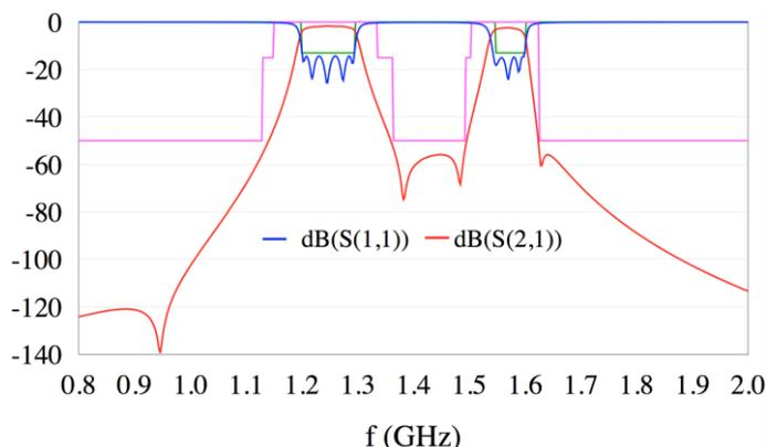
Figure 1. Ideal S Parameters of the filter for a quality factor ( $Q_0$ ) of 300.
