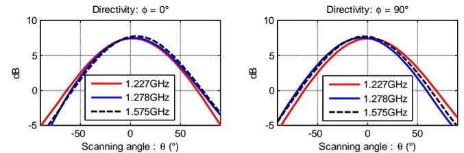
Fig. 4. Radiation patterns in two  $\phi$ -Planes for  $TM_{100}$  and  $TM_{300}$  modes.
