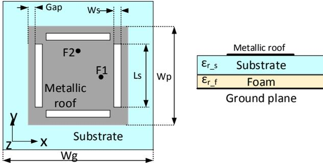
Fig. 1. Front view (left) and cut view (right) of the proposed structure of the dual-band GNSS microstrip antenna.
