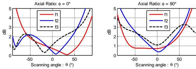
Fig. 5. Axial ratio for  $f_1=1.227$  GHz,  $f_2=1.278$  GHz and  $f_3=1.575$  GHz.
