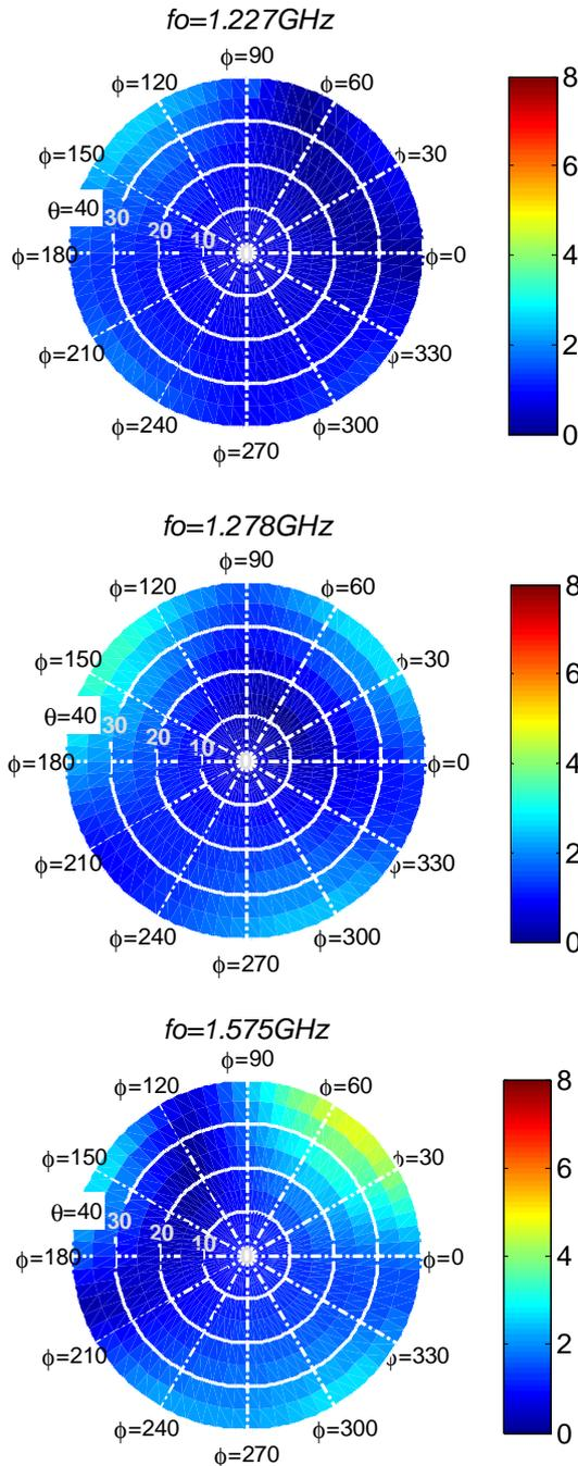
Fig. 6. Axial ratio for the three central frequencies of GNSS systems on 360 degree scanning angle ( $\theta_{max}=40^\circ$ ): L2 band ( $f_1=1.227$ GHz), E6 band ( $f_2=1.278$ GHz) and L1 band ( $f_3=1.575$ GHz).
