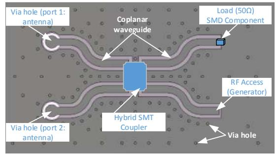
Fig. 2. Design view of the excitation circuit including the SMT hybrid coupler placement, the  $50\Omega$  SMD RF resistance and the RF access for feeding.
