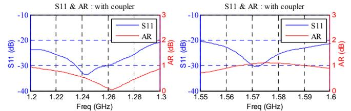
Fig. 3. Return loss and axial ratio with and without coupler for ( $\theta=0^\circ$ ;  $\Phi=0^\circ$ ).
