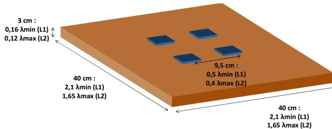
**Fig. 1.** Specified footprint of the 4 active antenna array
